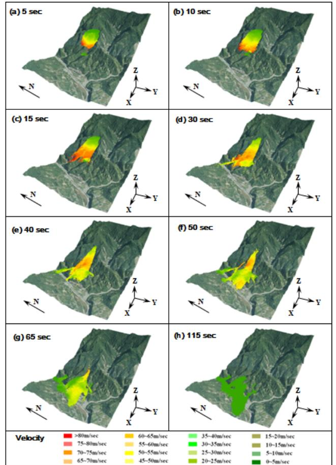
Figure 9 Diagrams the velocity and kinematic process of the Hsiaolin landslide.
