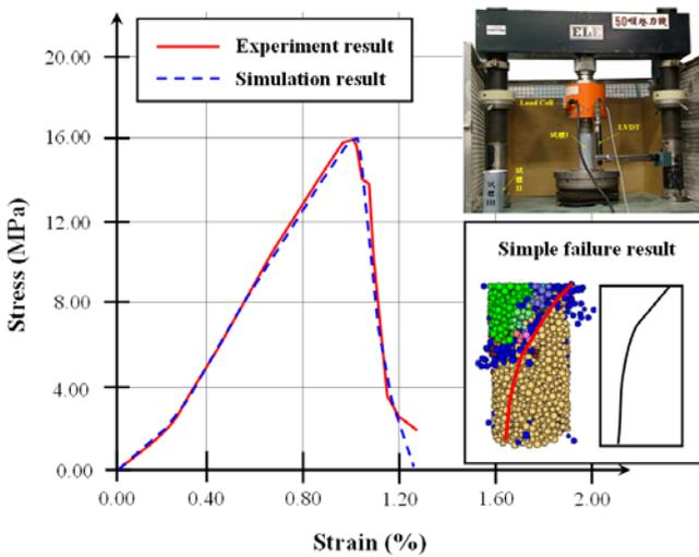
Figure 6 The comparison result of real and simulation uniaxial compression test.
