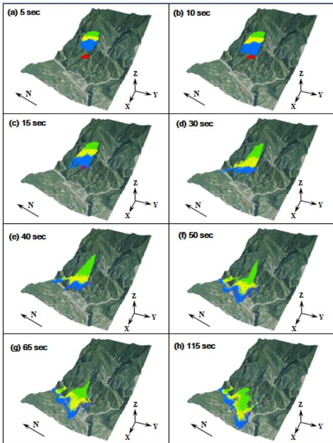
Figure 8 Diagrams kinematic process of the Hsiaolin catastrophic landslide. Blue color is the front part of the landslide mass, yellow color is the middle part, green color is the rear part, and red color is 590 Height.
