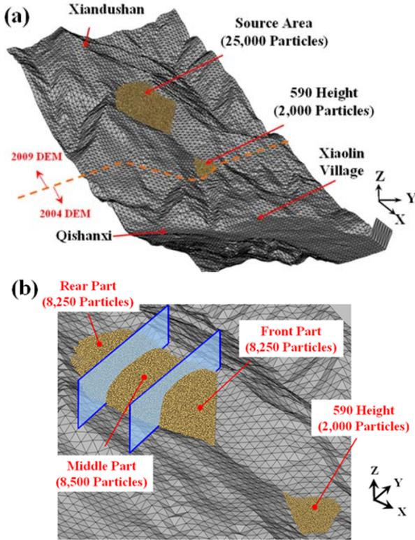
Figure 5 The Hsiaolin landslide modeling. (a) the sliding surface of the collapse area was constructed by 13,456 wall elements based on DEM data (after Morakot event), and the deposit area was used DEM data (before the Morakot event); and (b) diagrams the location of velocity measurement parts.
