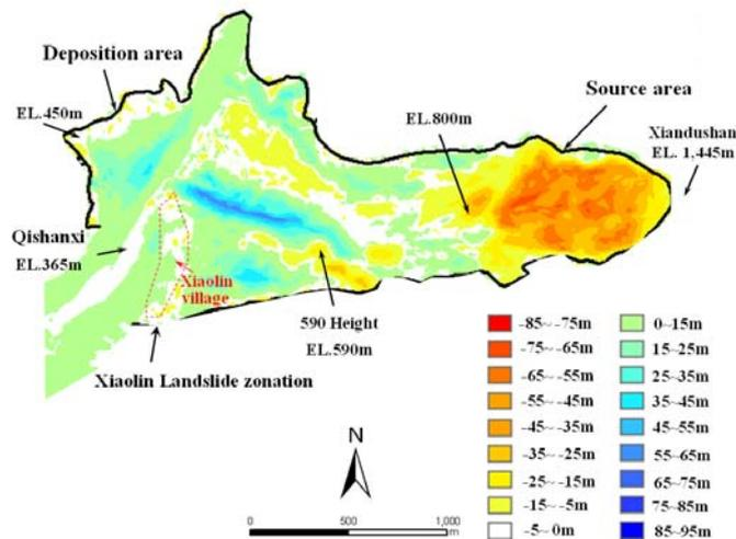
Figure 4 The result of DEM subtraction by 5m resolution between 2004 and 2009.
