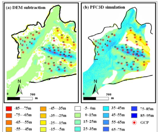
Figure 7 The comparison of simulation results: (a) 5 m resolution DEM subtraction between 2004 and 2009; (b) DEM subtraction by numerical simulation.
