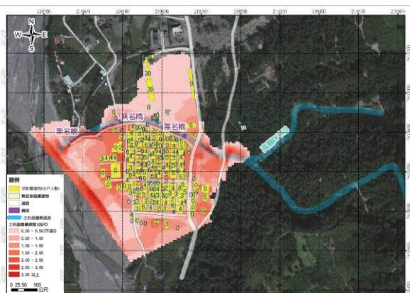
**Figure 6 200 years Kaohsiung City DF006 deposition depth diagram completed in 2010**
