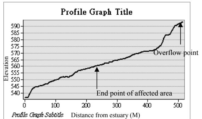
**Figure 2 Kaohsiung City DF006 stream longitudinal section elevation change diagram**
