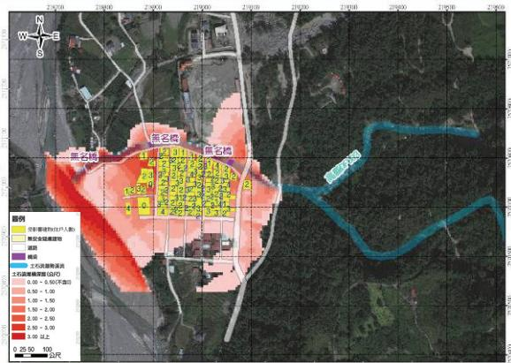
**Figure 5 200 years Kaohsiung City DF006 deposition depth diagram completed in 2008**
