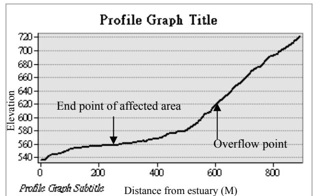
**Figure 3 Kaohsiung City DF068 stream longitudinal section elevation change diagram**
